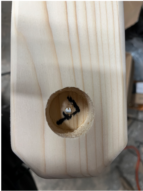
Pic 2. Each end of the beam is marked with its corresponding location on the frame.
