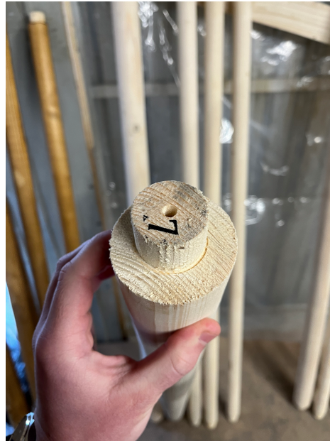
Pic 2. Each end of the beam is marked with its corresponding location on the frame.
